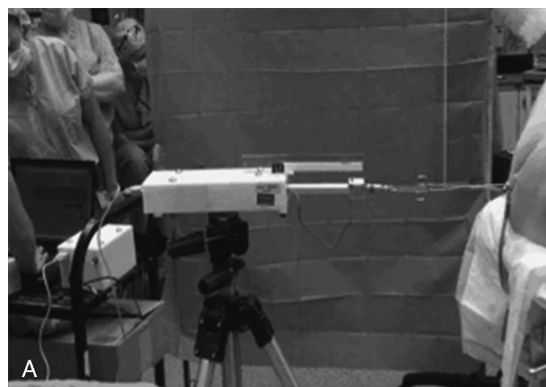
Figure 1a. A computer-controlled linear servomotor mounted on a tripod quantifying force-displacement behavior of the uterine cervix while applying caudally-directed tensile force to the handle of a tenaculum attached to the cervix. Figure 1b. Force-displacement graph demonstrating hyperelastic ramp curves for the 12 individual subjects. X-axis showing Cervix Location in mm based around the Hymen. Y-axis showing Force in N.
